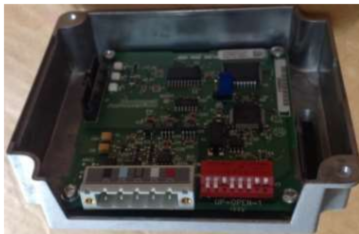
Figure 2-A 22-COMM-D DeviceNet Adapter in 22-XCOMM-DC –Base
