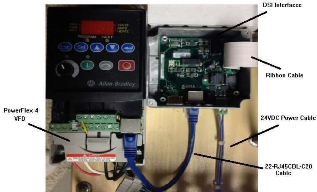
Figure 3-A DSI Interface Installed In 22-XCOMM-DC –Base
